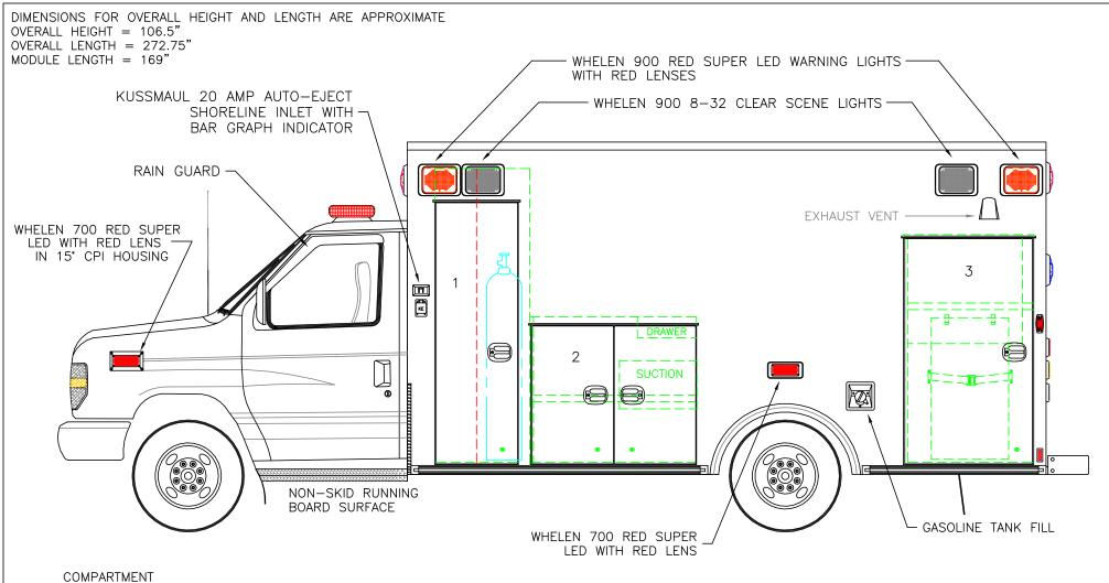
0.S.S #1 CLEAR OPENING: 68.00h x 18.25w INSIDE DIM'S.: 77.75h x 24.25w x 20.75d VERTICAL CENTER DIVIDER BACKBOARD/SCOOP STORAGE — FORWARD OXYGEN STORAGE — REARWARD
