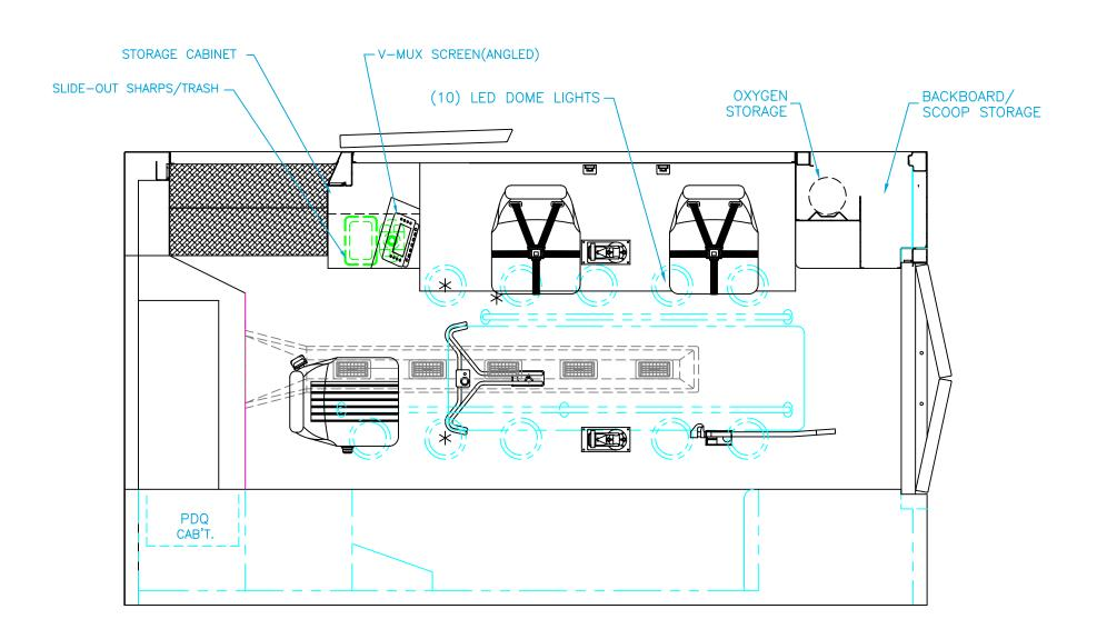
TWO (2) ANTENNA BASES LOCATED OUTBOARD OF DOME LIGHTS WITH COAX SERVICE LOOP
